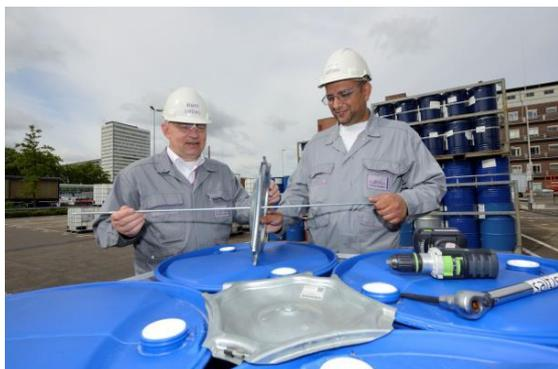
To secure loads, Saltigo GmbH uses special brackets that allow containers to be anchored securely on a chemical pallet. These not only withstand static tipping tests (lean tests) but also acceleration in dynamic driving tests.
