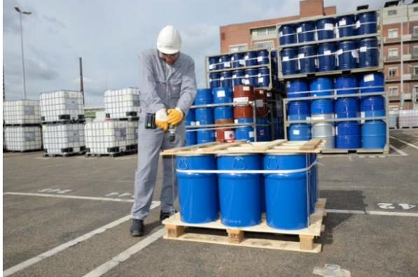
Smaller containers too can be stored together as a stable loading unit with the aid of boltings. Essential here is an even contact pressure that links the wooden structure with the pallet.
